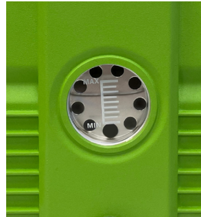
FIGURE 8: Sight glass, showing oil level
