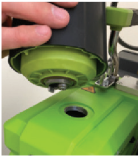
FIGURE 7: Demister removed, showing oil opening
